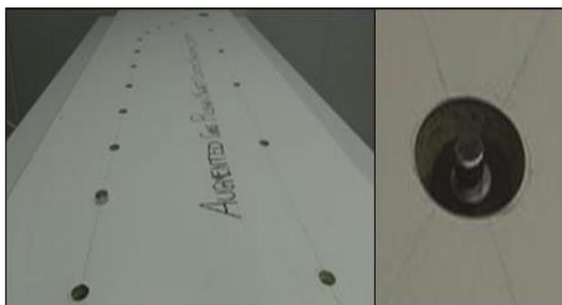
Figure 4. Magnet points' trail test bed.
