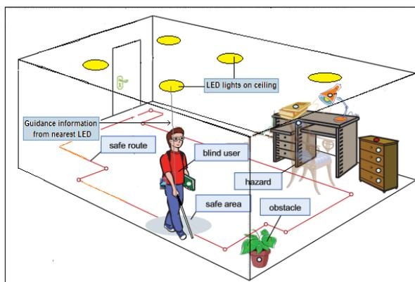
**Figure 7.** Visible light communication based smart grip indoor navigation system scenario.
