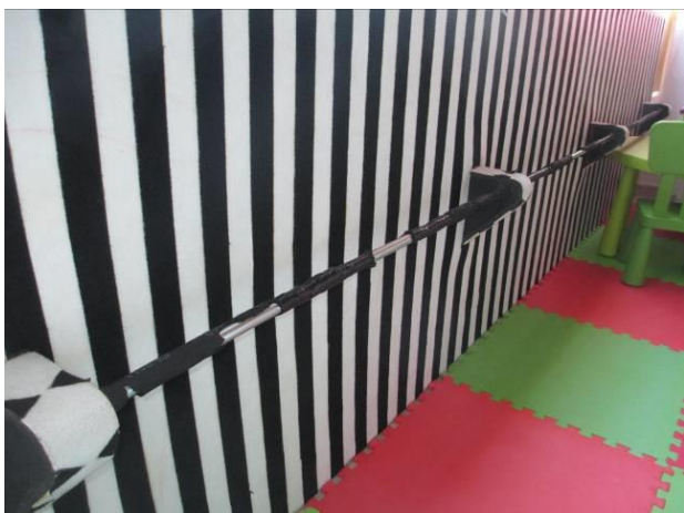
Figure 8. Ergonomic intervention as applied to a child's playroom. This view shows the wall coating of a special 'hook and loop' textile (for adjusting various toys) and of high contrast appearance. Moreover, a bar is fitted for balance purposes, and a soft floor tiles for safety.
