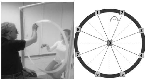
**Figure 3.** The experimental set-up. On the left, a visual impaired subject performing the task. On the right, the 8 points around the circumference are indicated. The diameter is 90 cm and the angle between two points is 45 degrees.
